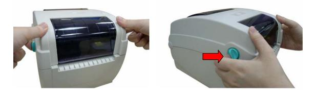
2. A top cover support at the rear of the printer will engage with lower inner cover to hold the printer top cover open.
