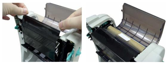
6. Turn the ribbon rewind gear until the ribbon plastic leader is thoroughly wound and the black section of the ribbon covers the print head. Close the ribbon access cover and the top cover.
