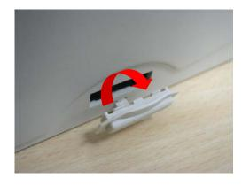
2. Plug in the SD card on main board.
