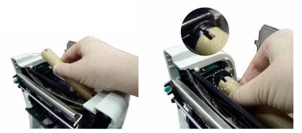
5. Stick the ribbon onto the ribbon rewind paper core.
