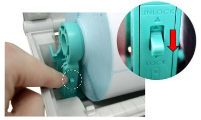
5. Place the paper, printing side face up, through the media sensor and place the label leading edge onto the platen roller. Move the media guides to fit the label width by turning the guide adjuster knob. Disengage the top cover support and close the top cover gently.
