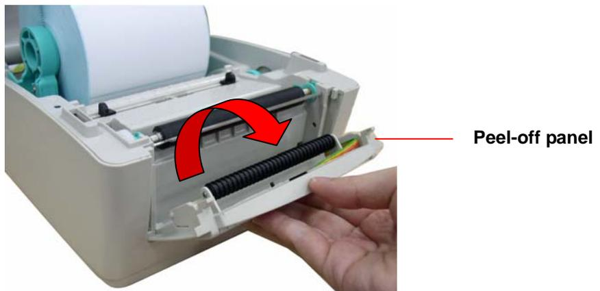
6. Lead the media through the backing paper opening, beneath the peel-off roller.
