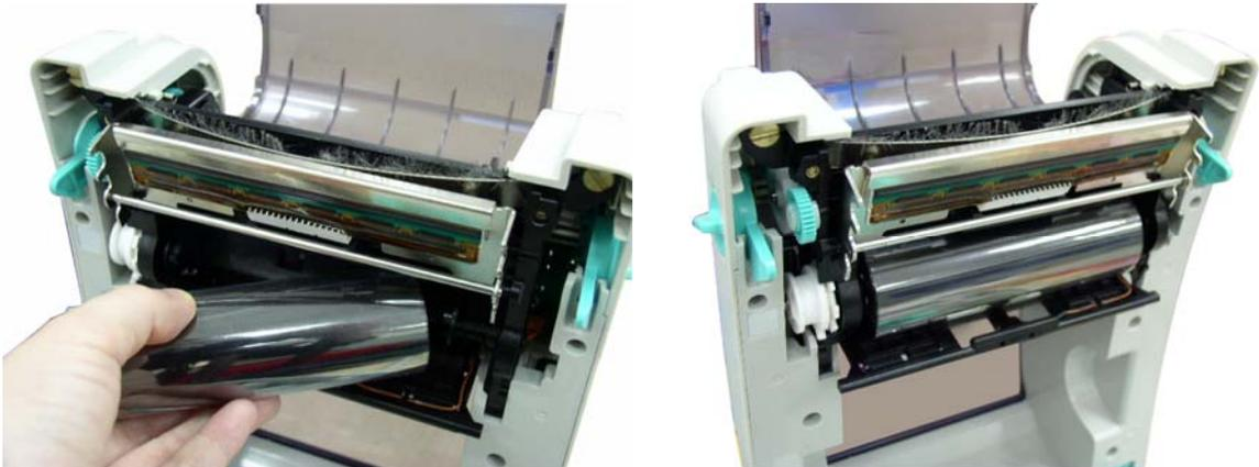
4. Insert the paper core right side onto the rewind hub. Align the notches on the left side and mount onto the spokes.
