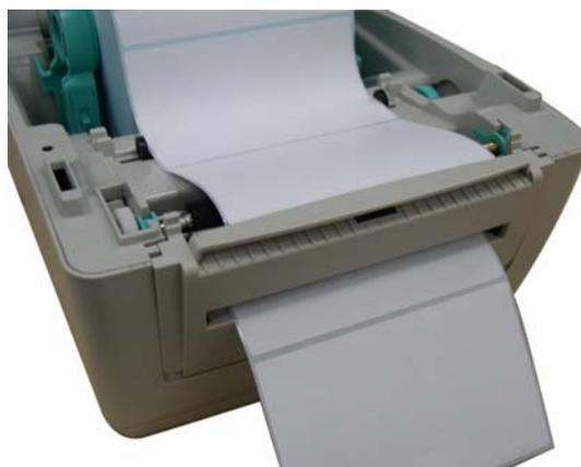
8. Disengage the top cover support and close the top cover gently.
