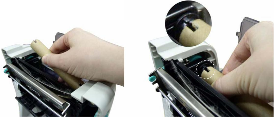
5. Stick the ribbon onto the ribbon rewind paper core.
