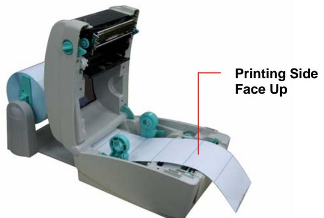
6. Move the media guides to fit the label width by turning the guide adjuster knob.
