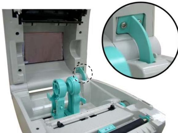
3. Hold the top cover and press the top cover support to disengage the top cover support with lower inner cover. Gently close the top cover.
