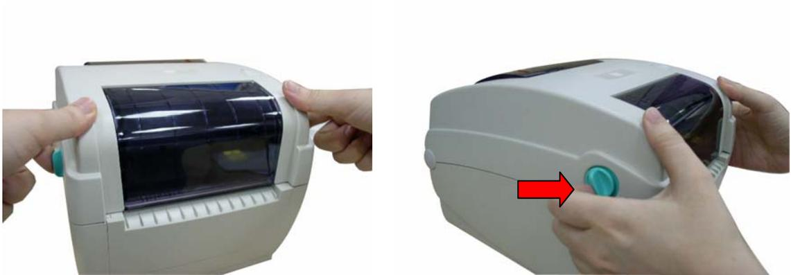
2. A top cover support at the rear of the printer will engage with lower inner cover to hold the printer top cover open.
