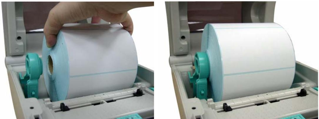
4. Press down the media holder lock switch to hold the label roll firmly.
